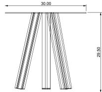
Paying homage to NY skyscrapers constructed by Mohawk ironworker's. The 13 table is designed to be quickly bolted together with ease. Constructed from a 1/4" round water jet cut Aluminum plate and 3 6061 Aluminum I beams, utility and beauty merge with ease.
